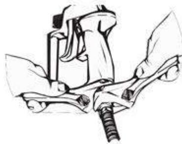
3. Remove filter from spray gun (refer to [Cleaning the Spray Gun Filter](#)).
