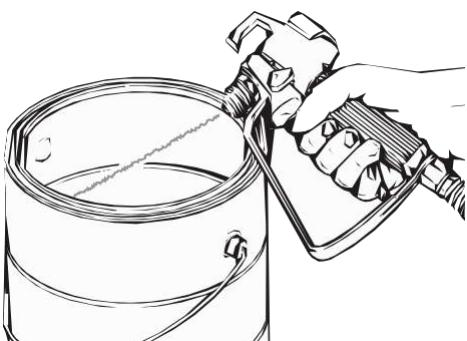
4. Release trigger. Turn the PRIME/SPRAY knob to PRIME. Turn the pump OFF (O). Trigger the gun into the waste container to be sure that no pressure is left in the hose.
