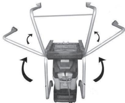
Turn the machine over onto its head. Pivot the legs upward, place the supplied wheel axle through the respective openings.
